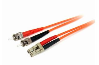
The FIBLCST7, 7-meter (23ft) Multimode 62.5/125 Duplex Fiber Patch Cable is terminated with one LC (male) connector and one ST (male) connector, to provide the necessary connection between fiber networking devices for high-speed, long distance networks.
